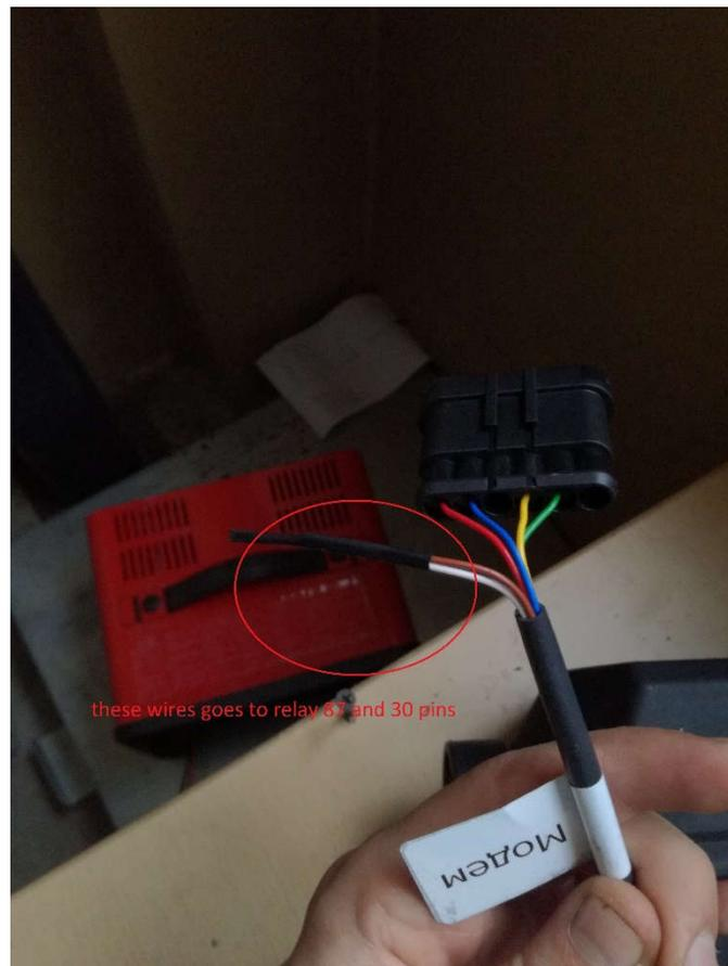
Those wires connects to "30" and "87" pins of relay
